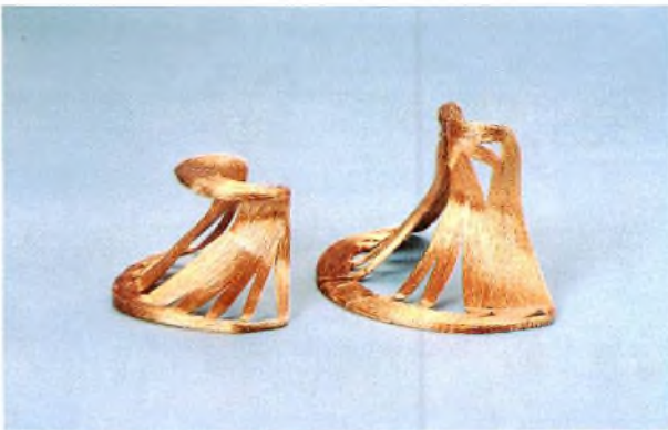
Fig.3 Saddle coils with flanges (left) and without flanges (right)
