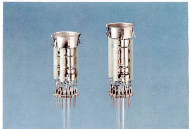
Fig.9 30AX gun (right) compared with 20AX gun (left)
